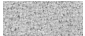
Acrylic Coated Galvalume ® (41) ☆ SR = 0.67 TE = 0.14 SRI = 56
